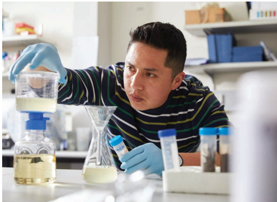
◀ Christian Cando-Dumancela filters soil samples to separate microorganisms, then ferments the extracts to grow the bacteria to sequence their genes.
